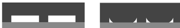
Figure 3-6: PDMS-based fluidic chip (Left), and the roof collapse in the fluidic channels (Right).
